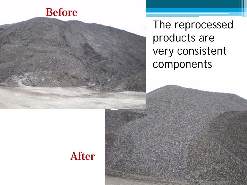
Fractionated RAP =Crushed and screened into different sizes
